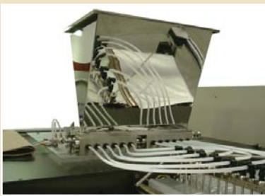
DCP - Feeder for watery, semi-dense and dense products like ketchup, mayonnaise, sauces, alcohol, etc.
