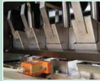
SSS - Feeder with oscillating movement for free-flowing powders and granules
