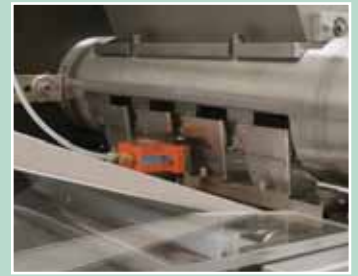
GPV - Feeder suitable for powders and granules (salt, pepper, sugar, 3 in 1, instant drink and similar)
