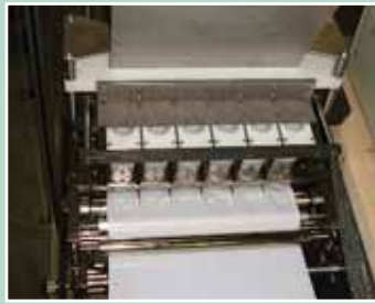
DTL - Volumetric linear cup doser for sugar coated pellets, small sweets, peanuts, etc.
