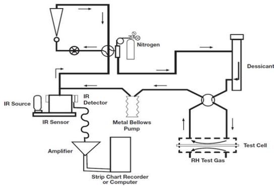
Figure 1. ASTM D3985.
