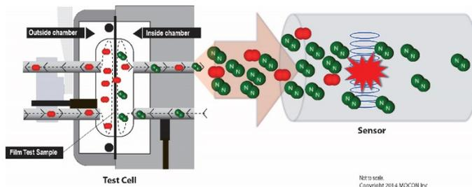
Figure 5. A test cell with a coulometric sensor.
