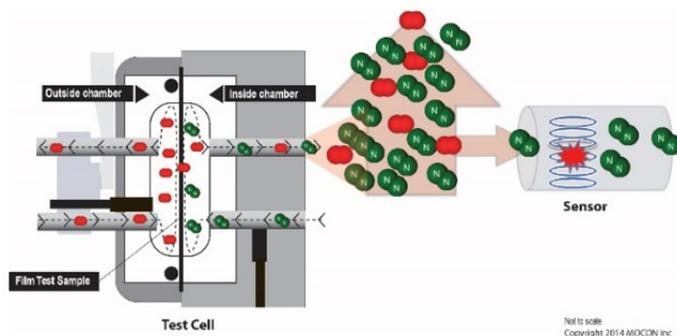
Figure 4. A test cell with a sensor that is not truly coulometric.
