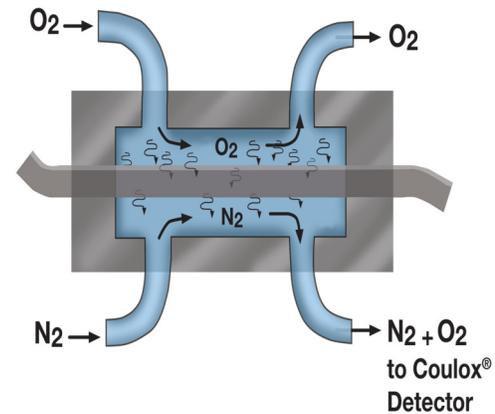
Figure 7. The setup for testing a film.
