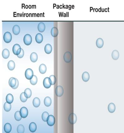
Figure 1. Permeation through a test barrier.
