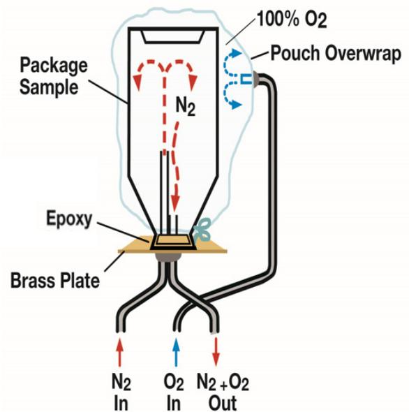
Figure 8. A setup for testing a package.
